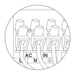
3 Correctly connect AC output wire in accordance with cable sequence and terminal position shown in the figure below. Please connect the ground wire at first, and then live wire and null wire. The ground wire is connected to the ground screw hold through O-type terminal.
