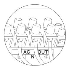
**Note:** The grounding wire shall be as thick as possible (cross-sectional area is not less than 4mm<sup>2</sup>). The grounding point shall be as close as possible to the solar storage inverter. The shorter the grounding wire, the better.
